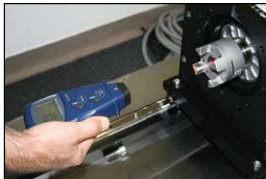
PT-130 recording rotational speed of machinery.
