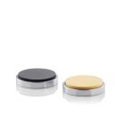
Reference elastomer blocks with DAkkS calibration certificate, single set/set of 3 or 6 Reference elastomer blocks can be used to check the indenter and measuring path of the hardness tester according to DIN ISO 48.
