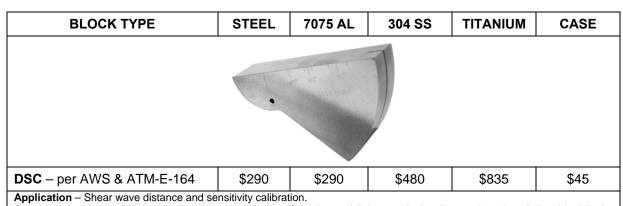
**Geometry** – 1" thick, 4" long with 1" radius and 3" radius. Contains a 3/8" deep x 1/32" radius notch and a 1/2" dia. side drilled hole for 45, 60, & 70 degrees.
