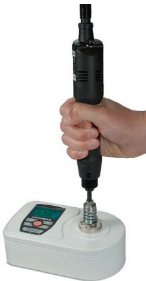
Fig. 2 Proper use of a rundown fixture with a motorized torque tool. Note the axial vertical alignment.
