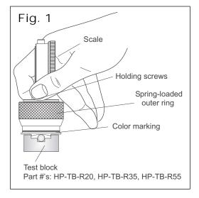
**NOTE:** Do not loosen the holding screws of the movement under any circumstances. Loosening these screws may alter the calibration of the instrument.
